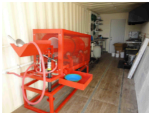
Lab Dirty Section with Spiral Finisher
