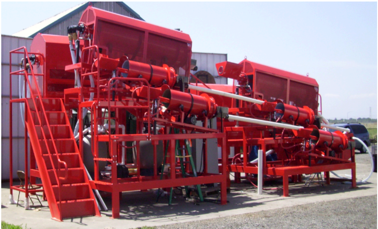
10T/HR Hard Rock Concentration Circuit (HRCC-10)
