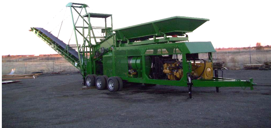
100 Yd 3 /Hr Mobile Placer Plant (MPP-100)
