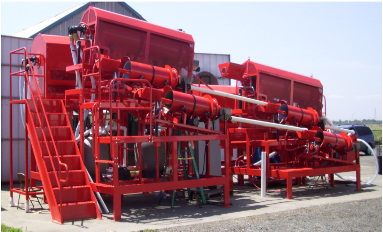
10T/HR Hard Rock Concentration Circuit (HRCC-10)
