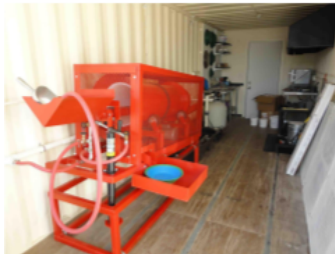
Lab Dirty Section with Spiral Finisher
